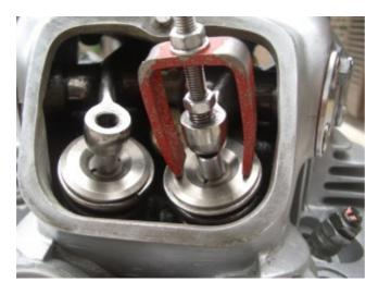
Compress the valve spring. If the retainers stick a little, a tap on the spring collar will break them loose. Continue compressing until you can remove the two retainers. A magnetic screwdriver or a pair of fine tweezers is handy for picking out the retainers.
