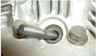
It needs to be a minimum of 6 cm (2.5") long and the lip must stick out about 8-9 mm (3/8") Cut a slot in the top of the bolt in line with the lip. Chamfer one end and mark the orientation of the lip with a dab of paint. The bolt must be a nice sliding fit in the plug.
