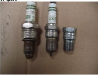
Knock out the ceramic and centre electrode (wear eye protection!) and drill out. I found it really hard to remove the ceramic centre and so used a TDC finding tool, enlarging the central hole to accept the bolt.
