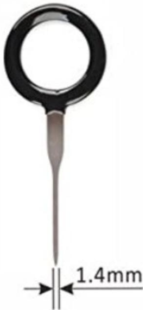
Insert the extractor from the wire side of the connector, between the connector body and the yellow seal, on the lock side of the connector. Ensure that the extractor goes straight in. Gently work the extractor until the lock releases and the wire/pin assembly extracts without excessive force.
