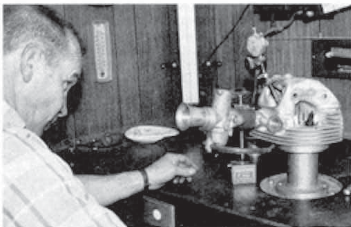
Jerry Branch, of Branch Flowmetrics, carefully checks the inlet valve opening while flow testing the factory-recommended modification using the 36mm Amal Concentric carburetor.
