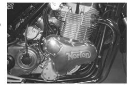
• Cut double eared clip off oil cooler, cut double eared clip off oil tank, and remove hose.
