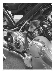
• Remove oil pump banjo bolt, cut double eared clip off oil cooler, and remove hose 6100036.
